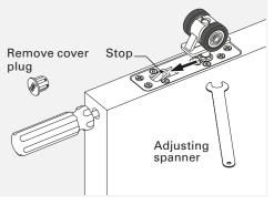
Keep the screwdriver in place while using the spanner to slide the hanger pin sideways.
