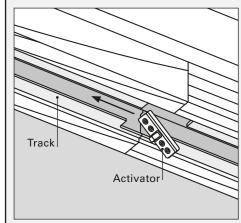
NOTE: If you have a Fixed Head Jamb and have screwed through the track you will need to remove some screws to insert the activator. Reinsert when SofStop installation is complete.
