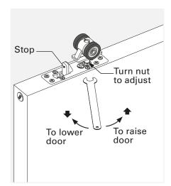
Note: The top of the hanger pin screws into a self-locking Nyloc type nut in the carriage. For the assembly to remain in its adjusted position over time the hanger pin must be screwed into the nylon locking portion of the nut by at least 3 full turns.
