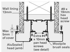
AluSealed head jambs longer than 1 metre require an extra screw to hold the centre of the jamb to the bottom of the track as shown. Spot through the pre drilled hole in the flange with a ø2.5mm drill into the bottom of the track.
