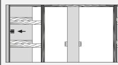
Position the distance setting tool inside the back stud and gently open the door onto it. The activator will slide along the track into the correct position. The rear activator is now positioned. Securely tighten all four grub screws.
